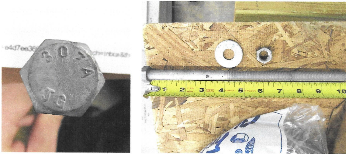
Figure 5: Example of a Bolt, Washer, and Nut Received from the Client
