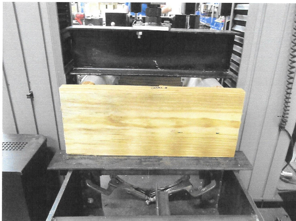
Figure 15: Test Setup Viewed from the Support Side and Showing the Load Application Beam
