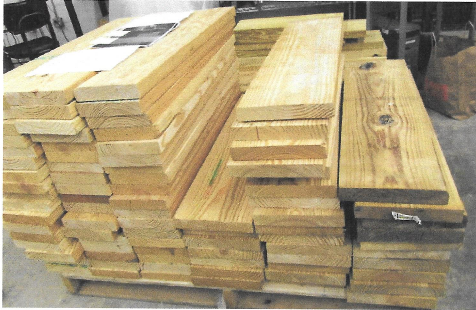
Figure 9: Lumber Received from the Client Note: Not every piece contained a grade stamp.
