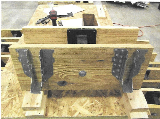
Figure 10: Constructing a Configuration 1 Specimen
