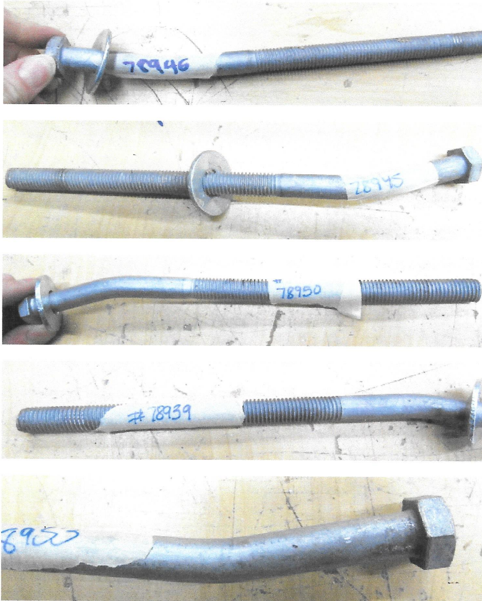
Figure 19: Examples of Bent Bolts Removed from Assemblies after Testing
